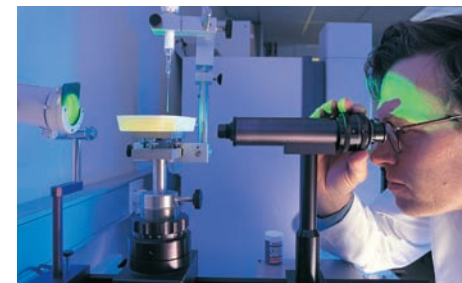
"Dr. Wax" Leif Axell Torgersen measures contact angles between water and wax.
